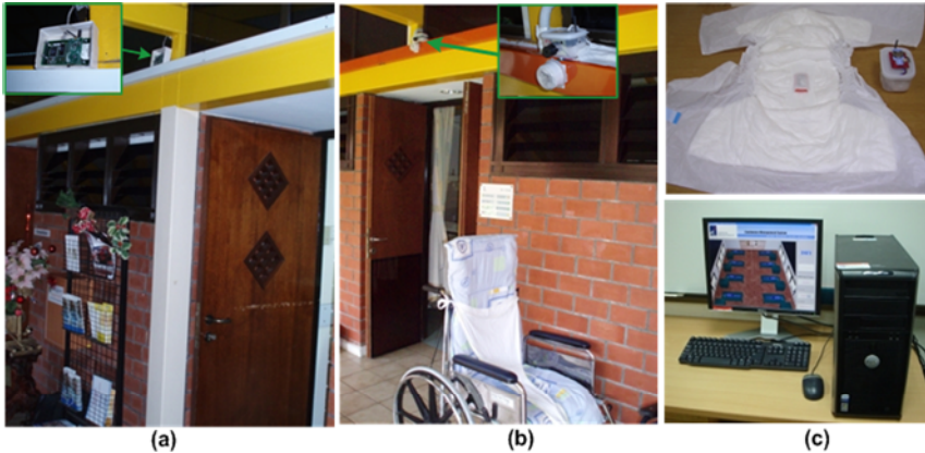
Fig. 3. SCMS deployment at Nursing Home: (a) Gateway Node (Service Unit) (b) Relay/Actuator Node (Relay Unit) (c) Top: Wetness Sensor (Sensor Unit) and Diaper Node (Intelligent Unit), Bottom: UI System (Service Unit)
