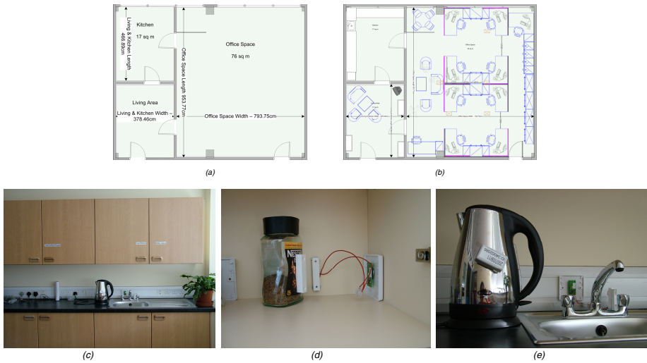
Fig. 2. Overview of the smart environment used for testing (a) plan view of entire room layout showing split between the kitchen and living area and a research desk based area (b) detailed design view of entire room layout (c) picture taken within the kitchen environment (d) picture of coffee jar with the sensor (e) picture of kettle and water tap with the sensors
