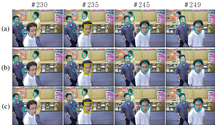
Rectangle: Face detected initially by the detection process [9] Ellipse: Face tracked by the tracking process after detection
